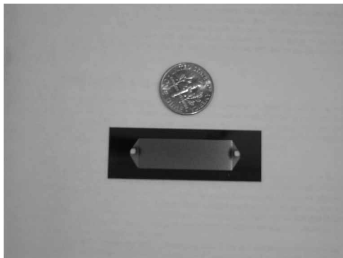
Figure 1. Top view of silicon microseparator.
